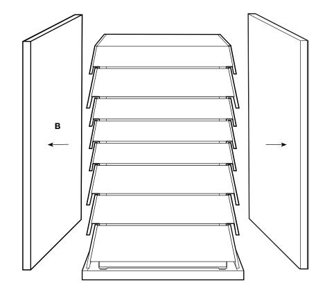
3. 2 people at the base and 1 supporting the top of the piece to prevent tipping. Carefully lift from under the bottom white drawer panels (C).
