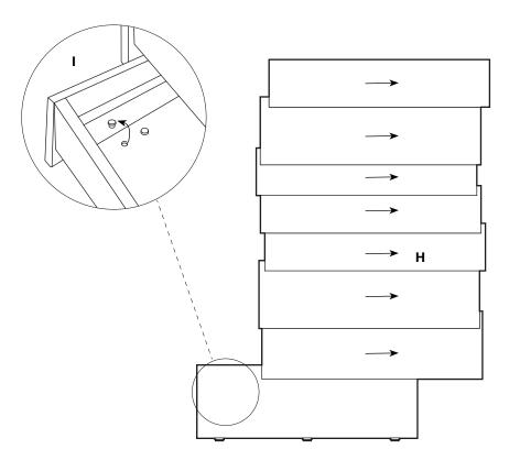
6. Using a flat-head screwdriver, turn CLOCKWISE to lower the castor wheels (J). Turn each wheel the same number of turns to ensure stability. NOTE. Only extend enough to allow the unit to move freely on the floor. DO NOT extend the castors fully as they will leave their housing. The screwdriver must be large enough to drive in an M10 screw.
